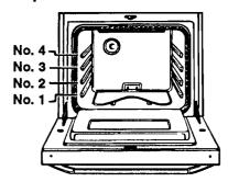
Your oven has two racks. One rack is straight and the other is offset (raised). The shape of the offset rack helps you space racks better.
